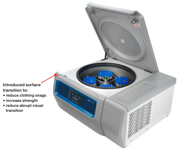
Figure 2: New door shape and open angle provide a reach area closer to the user than the previous design. Grip area for open door position is lower and closer to the user.
